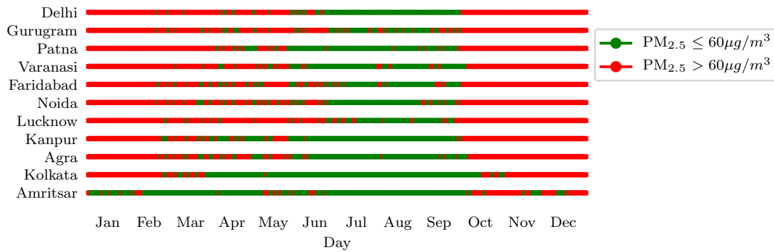
Figure 4: Violation of daily India limit of PM_{2.5} level ( 60 \mu g/m^3 ) by eleven cities in the IG plain over the year. Most of these cities (except Amritsar and Kolkata) violated India's limit across the year except a few months (monsoon season); hence air pollution is a year-long problem for most cities in the IG plain. Note that the time-span of PM_{2.5} data of all cities is from April 2018 to April 2021 (common time period based on the availability of PM_{2.5} data of all cities) which is averaged out along same day to show the readings over the year.
